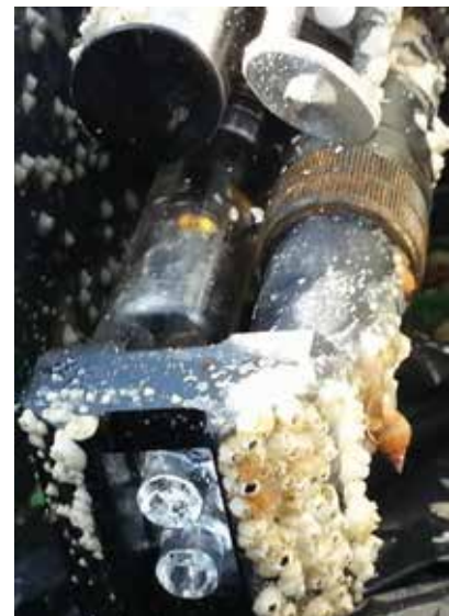
Clean sensor faces after nine months in-situ. (Image courtesy of Adrian Round, Director of Observatory Operations, Ocean Networks Canada)
