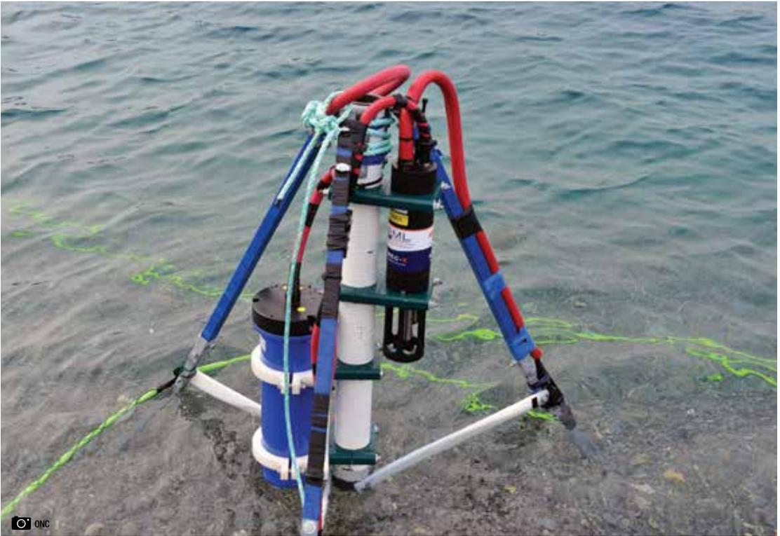
Figure 2: Gascoyne Inlet Remote Cabled Observatory with AML Oceanographic instrument and UV antifouling system.
